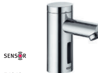
SENSOR 54912 Infrared basin mixer without pop-up waste, 1-hole installation, modular monoblock without base, infrared sensor (automatic settings), adjustable flow timer (mains operation 230 V)
