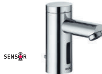
SENSOR 54911 Infrared basin mixer with/without pop-up waste, 1-hole installation, modular monoblock without base, infrared sensor (automatic settings), adjustable flow timer (battery 6 V lithium DL 223 A)
