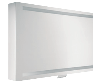
Mirror cabinet 1 lift up door Body: aluminium, silver anodized Lighting: • Fluorescent lamps (2 x 21 W T5) Features: • Mirrors on the sides • 1 light switch (on the outside) • 2 interior electric sockets • 1 exterior electric socket • 1 adjustable interior mirror (200 x 520 mm) • 5 variably adjustable glass shelves Dimensions (w x h x d): 950 x 650 x 160 mm
