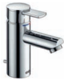
Single lever washbasin mixer with/without pop-up waste, 1-hole installation, ceramic cartridge with temperature limiter
