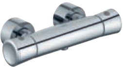
Thermostat battery for shower for on wall mounting, handle with 50% quantity limiter, safety cut-off at 38°, intrinsic protection against backflow
