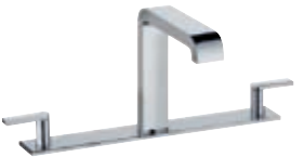
Three-hole basin mixer Model with plate, depth gauge 200 mm with/without pop-up waste, depth gauge 300 mm with pop-up waste, 3-hole installation, 90° head parts with ceramic sealing gaskets
