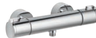
Thermostat battery for shower exposed fitting, handle with 50% quantity limiter safety cut-off at 38°, intrinsically safe against backflow
