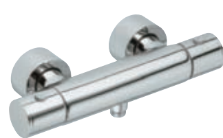
Thermostat battery for shower for on wall mounting, handle with 50% quantity limiter, safety cut-off at 38 °C, intrinsically safe against backflow
