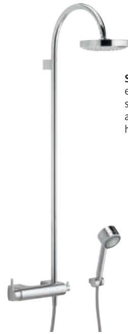
Single lever bath tub mixer with head shower exposed fitting, cartridge mixer with ceramic sealing gaskets, with automatic return bath tub/shower, head shower swivelling, Ø 180 mm, hand shower with normal-, soft-, and massage jet, with sliding bracket for hand shower and shower hose (2000 mm)
