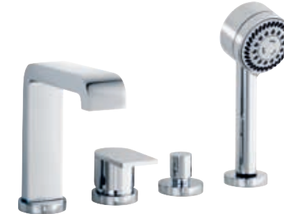
Single lever bath tub and shower mixer 4-hole bath tub edge installation, ceramic cartridge with temperature limiter, with automatic return bath tub/shower, concealable hand shower
