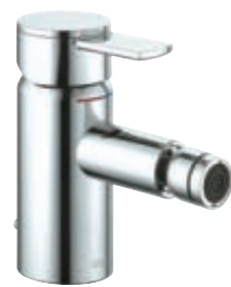
Single lever bidet mixer with pop-up waste, 1-hole installation, ceramic cartridge with temperature limiter
