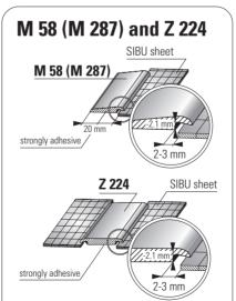
Strongly adhesive edge or middle profile with dimensions of  $2,705 \times 22$  mm (M 287:  $2,705 \times 28$  mm). These profiles are suitable for both absorbent and non-absorbent surfaces, whereby a non-absorbent surface is recommended.
