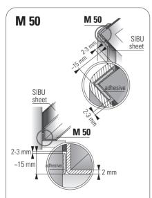
Non-adhesive, flexible interior and exterior corner profile with dimensions of  $2,705 \times 50$  mm. Stick the corner profile onto the underlying surface with adhesive.
